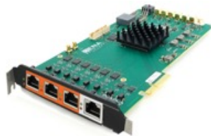
Odin-Z1-3S-6P-1T-RT45 has native 1000BASE-T1 and 100BASE-T1 interfaces for testing automotive Ethernet.
