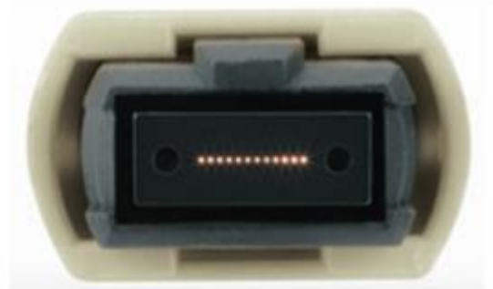
Figure 3: 12 fiber ends in an MPO12 connector
