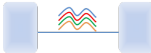
Figure 2: A single fiber between devices – several wavelengths are used
