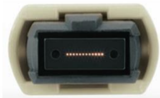
Figure 3: 12 fiber ends in an MPO12 connector
