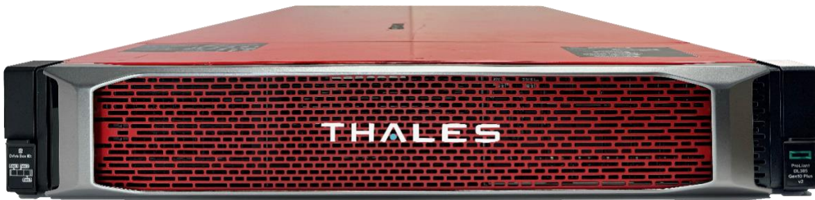
Figure 1: The Thales CYBELS RTG, 19" rack mounted version.
