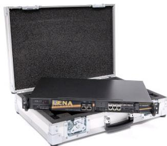
*A smart, robust flightcase is available for the ValkyrieCompact. It features customized padding and is ideal for protecting the tester during transportation.*
