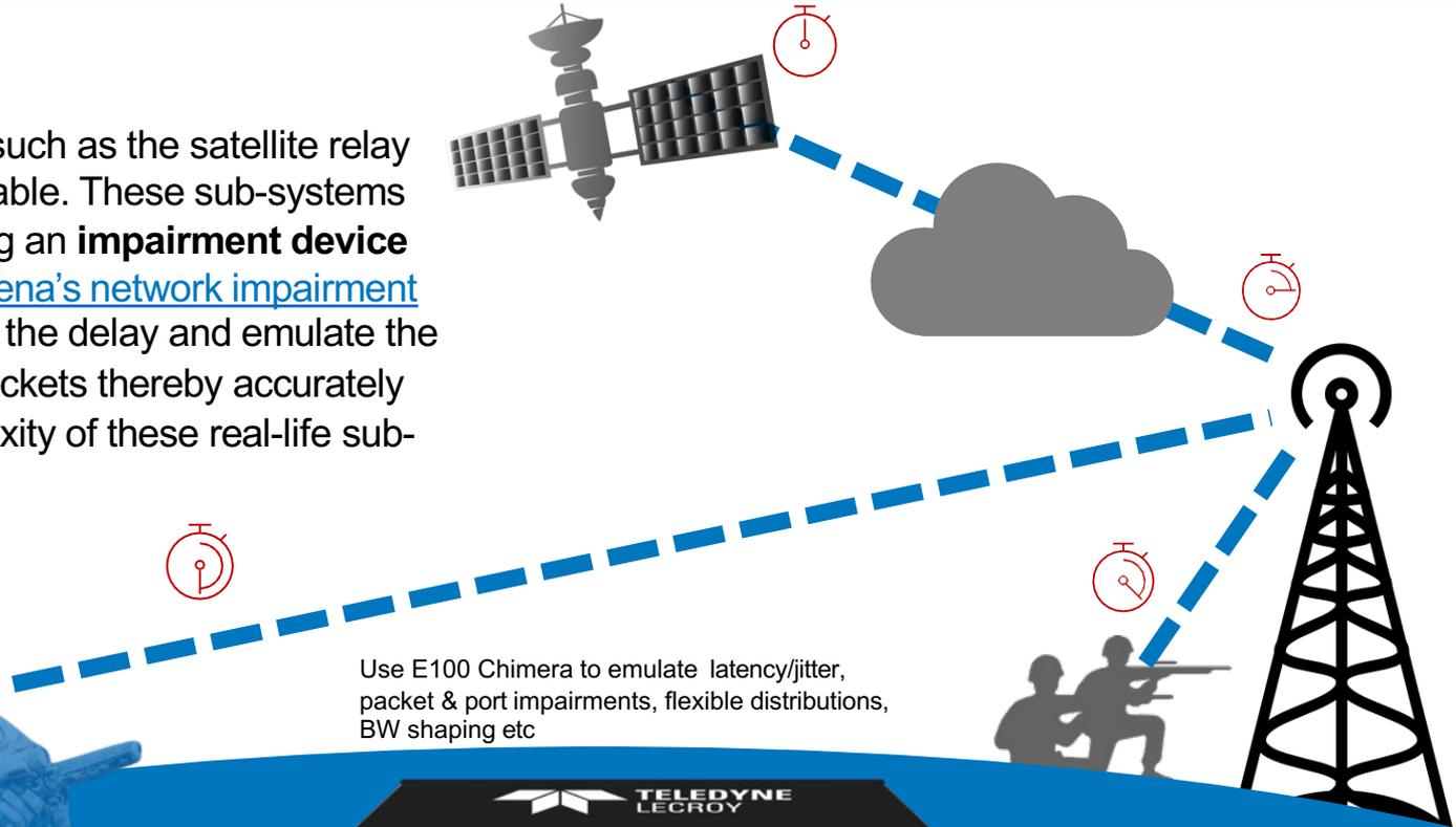
Use E100 Chimera to emulate latency/jitter, packet & port impairments, flexible distributions, BW shaping etc
